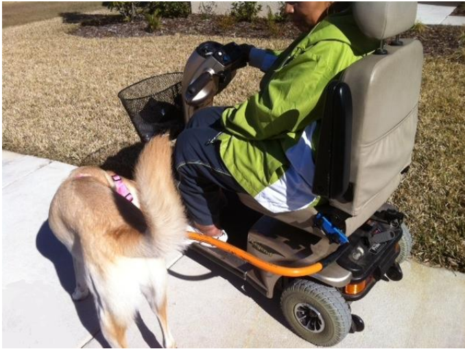
Clamp to Seat Hinge on Pride Legend Scooter Adjusted to Dog's Shoulder Ht.
