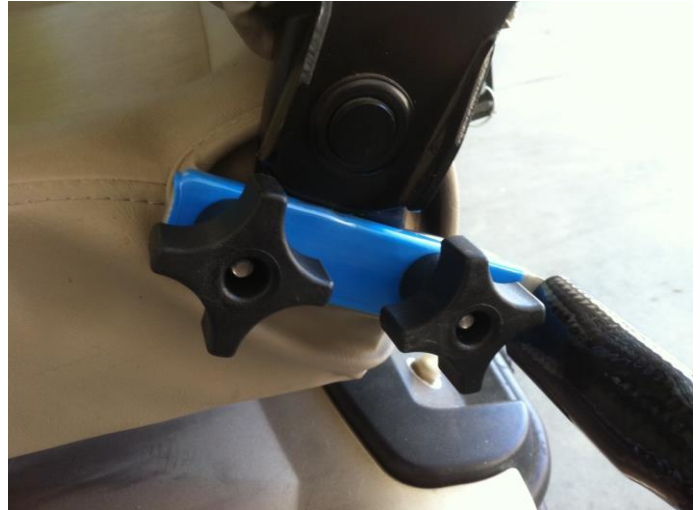
Close-up Pride Legend BTL Mounted to Seat Hinge Angled back to Locate BTL as far aft as possible
