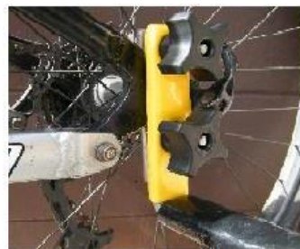
Bolts Above & Below Clamping Axle Mount Against Rear Axle
