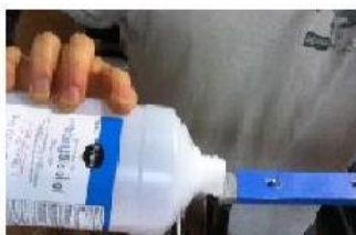
Pour Alcohol into Coupling. Repeatedly Tilt & Rotate BTL So All Coupling Inner Surfaces Are Soaked. Wait 5 minutes Then Forcibly Rotate Coupling.
